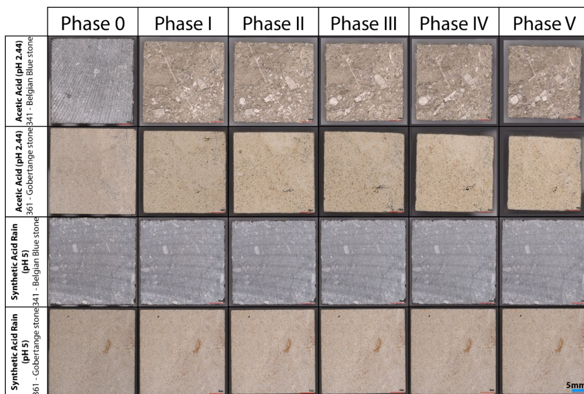
Figure 2 - Appendix. Mapping and evolution of surface finishes following the test phases. There is a noticeable reduction in the size of the samples and a change in texture for both stones following immersion in an acetic acid solution. The surface almost does not change when immersed in a synthetic acid rain solution.
